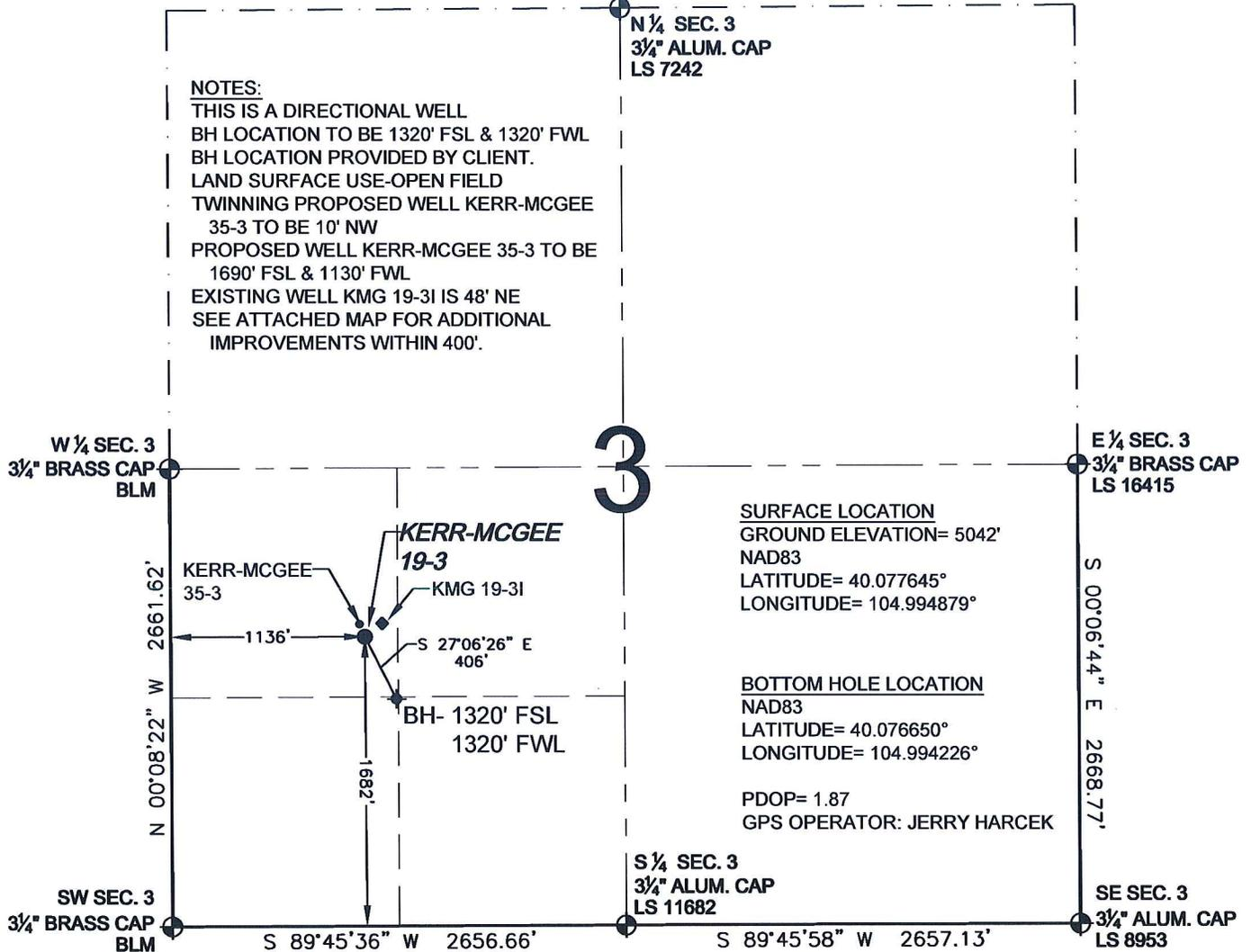
WELL KERR-MCGEE 19-3 TO BE LOCATED 1682' FSL AND 1136' FWL, SECTION 3, T1N, R68W OF THE 6th P.M.
