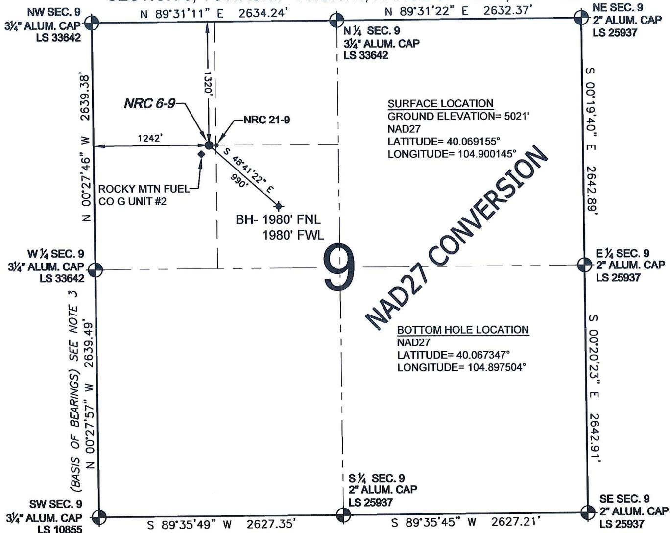
WELL NRC 6-9 TO BE LOCATED 1320' FNL AND 1242' FWL, SECTION 9, T1N, R67W OF THE 6th P.M.
