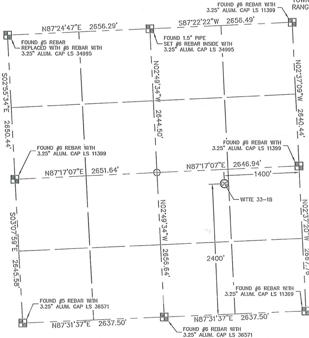
In accordance with a request from Dan Casper with Noble Energy Inc. King Surveyors Inc. has determined the surface location of the WITTE 33-1B to be 2400' from the SOUTH line and 1400' from the EAST line as measured at right angles from the section line of Section 1, Township 2 South, Range 45 West of the Sixth Principal Meridian, County of Yuma, State of Colorado.
