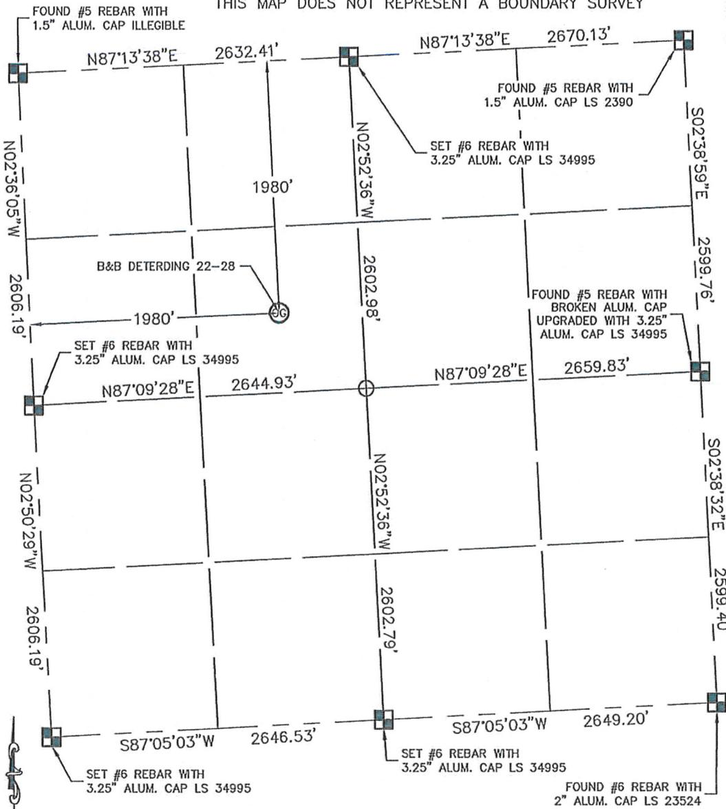
In accordance with a request from Dan Casper with Noble Energy Inc. King Surveyors Inc. has determined the surface location of the B&B DETERDING 22-28 to be 1980' from the NORTH line and 1980' from the WEST line as measured at right angles from the section line of Section 28, Township 1 South, Range 44 West of the Sixth Principal Meridian, County of Yuma, State of Colorado.
