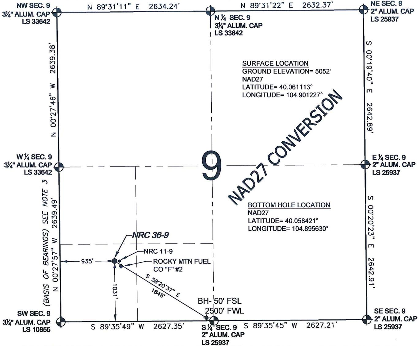
WELL NRC 36-9 TO BE LOCATED 1031' FSL AND 935' FWL, SECTION 9, T1N, R67W OF THE 6th P.M.
