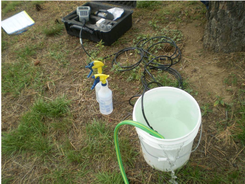
Photo #1 Purging the well while taking parameter readings
