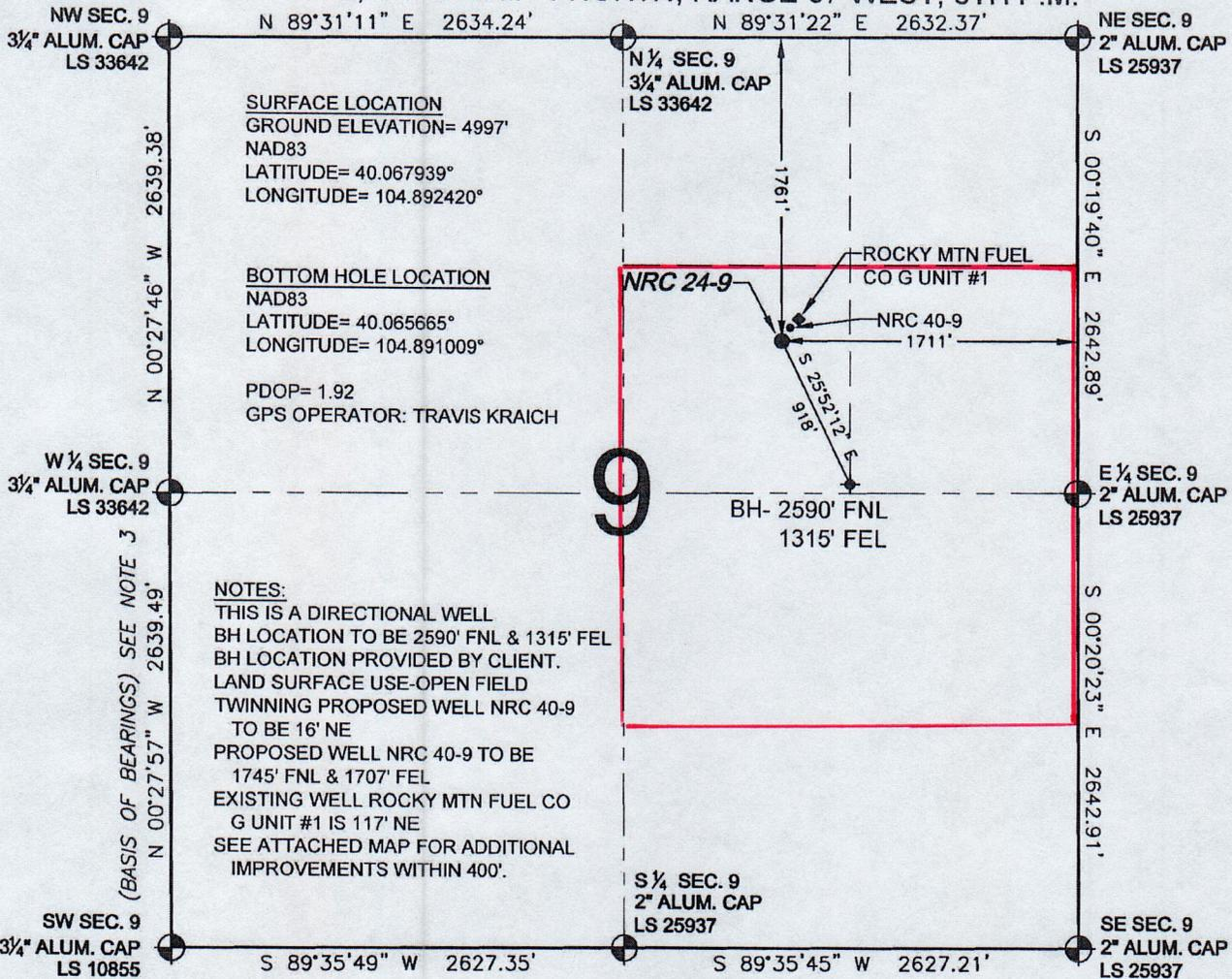
WELL NRC 24-9 TO BE LOCATED 1761' FNL AND 1711' FEL, SECTION 9, T1N, R67W OF THE 6th P.M.
