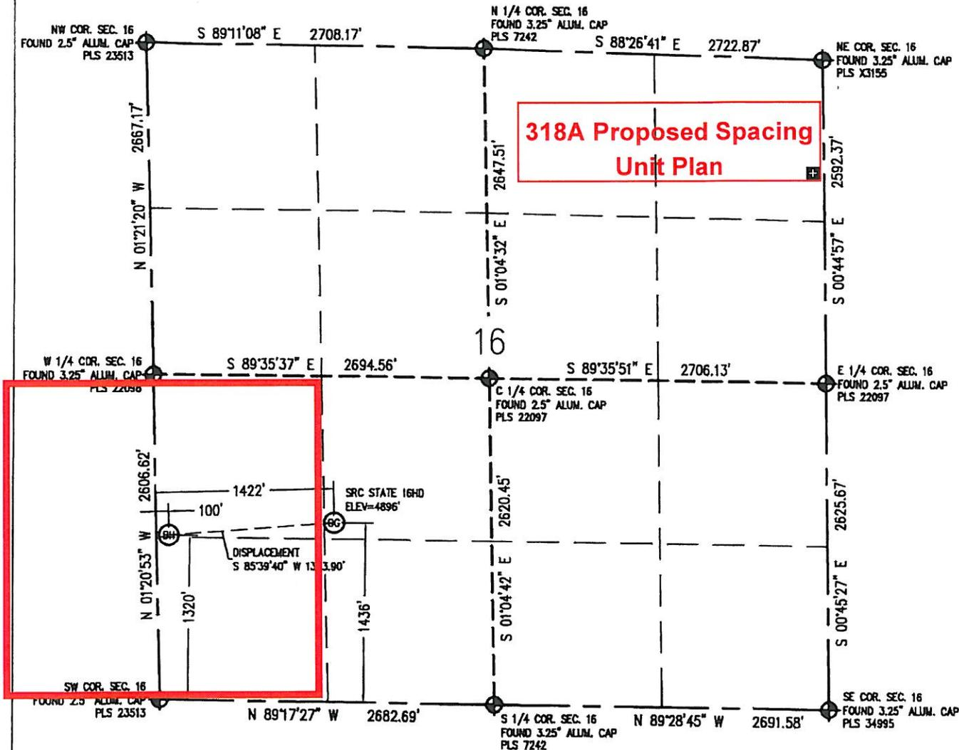
IN ACCORDANCE WITH A REQUEST FROM CRAIG RASMUSON - SYNERGY RESOURCES, BASELINE ENGINEERING CORP. HAS DETERMINED THE LOCATION OF THE SRC STATE 16HD TO BE 1436' FSL AND 1422' FWL, AS MEASURED AT NINETY (90) DEGREES FROM THE SECTION LINE OF SECTION 16, TOWNSHIP 4 NORTH, RANGE 67 WEST AND THE BOTTOM HOLE LOCATION TO BE 1320' FSL AND 100' FWL OF SECTION 16, TOWNSHIP 4 NORTH, RANGE 67 WEST, 6TH PRINCIPAL MERIDIAN, WELD COUNTY, COLORADO.
