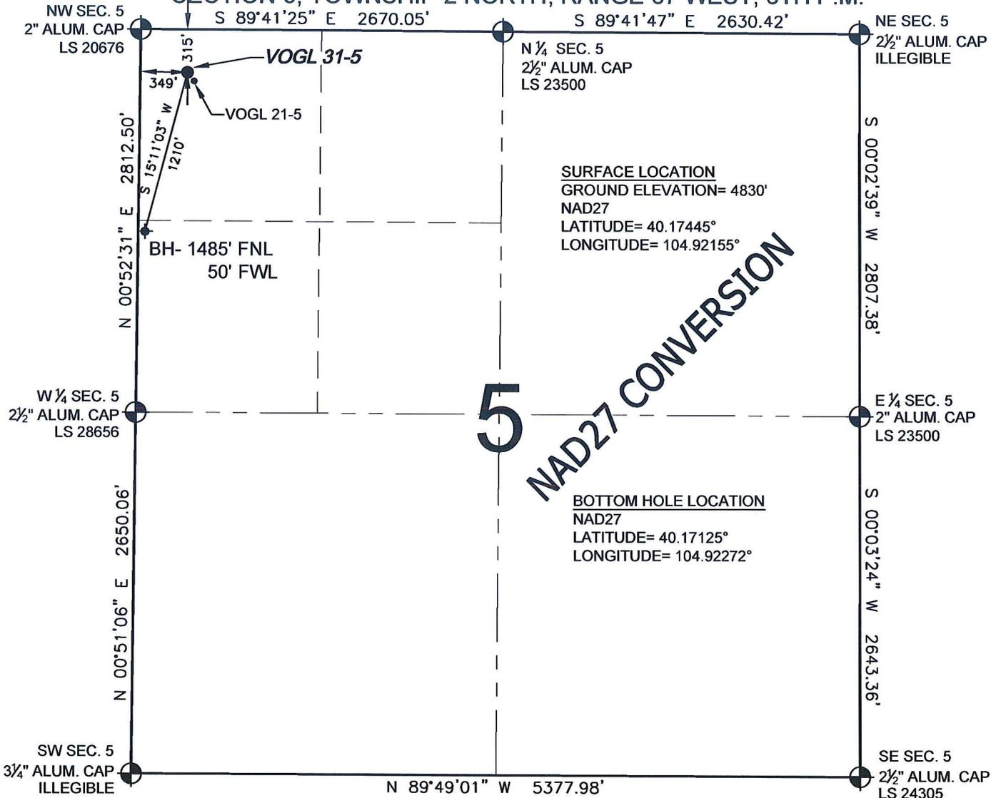
WELL VOGL 31-5 TO BE LOCATED 315' FNL AND 349' FWL, SECTION 5, T2N, R67W OF THE 6th P.M.
