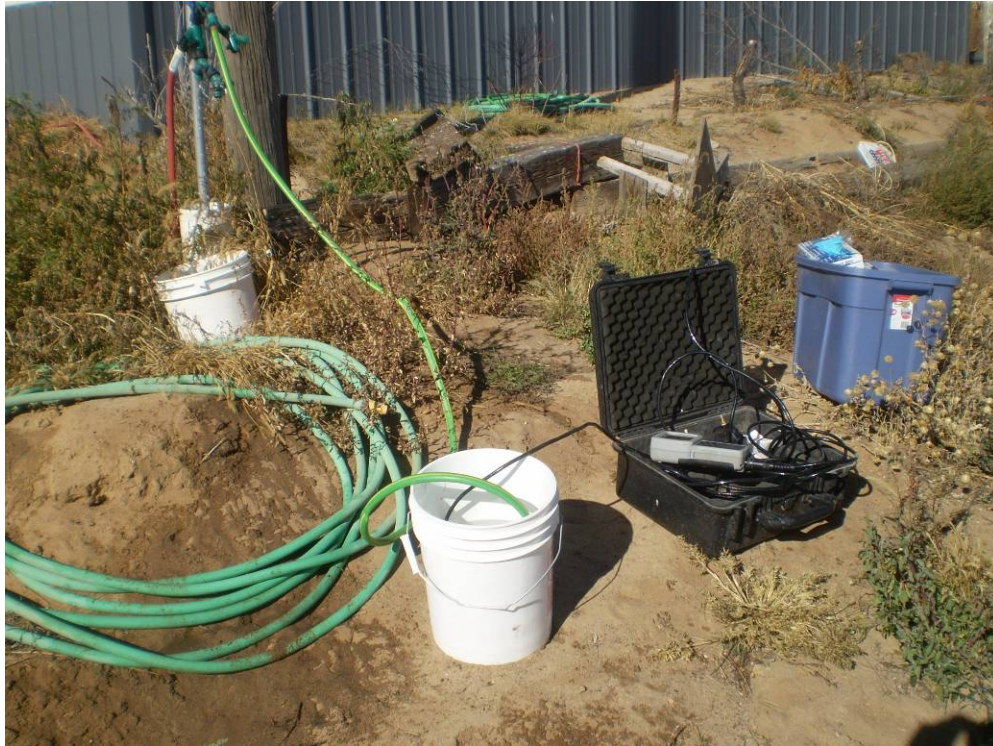
Photo #2 View of the purging process including the collection of parameters
