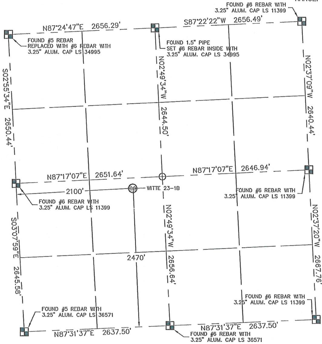
In accordance with a request from Don Casper with Noble Energy Inc. King Surveyors Inc. has determined the surface location of the WITTE 23-1B to be 2470' from the SOUTH line and 2100' from the WEST line as measured at right angles from the section line of Section 1, Township 2 South, Range 45 West of the Sixth Principal Meridian, County of Yuma, State of Colorado.
