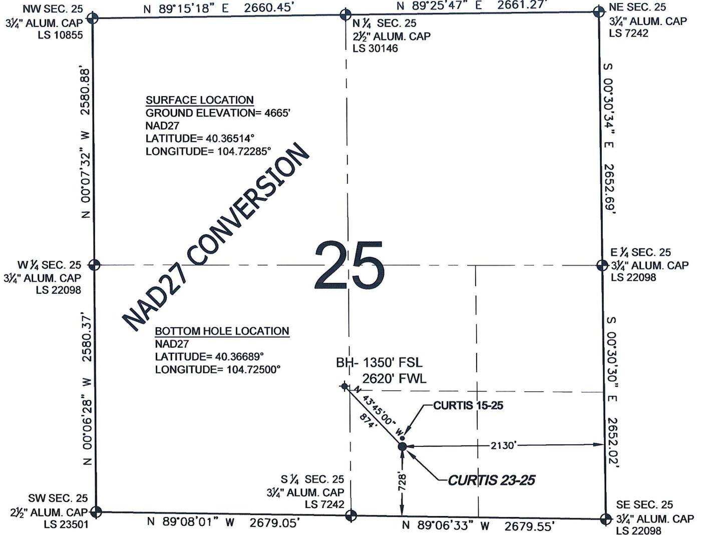
WELL CURTIS 23-25 TO BE LOCATED 728' FSL AND 2130' FEL, SECTION 25, T5N, R66W OF THE 6th P.M.
