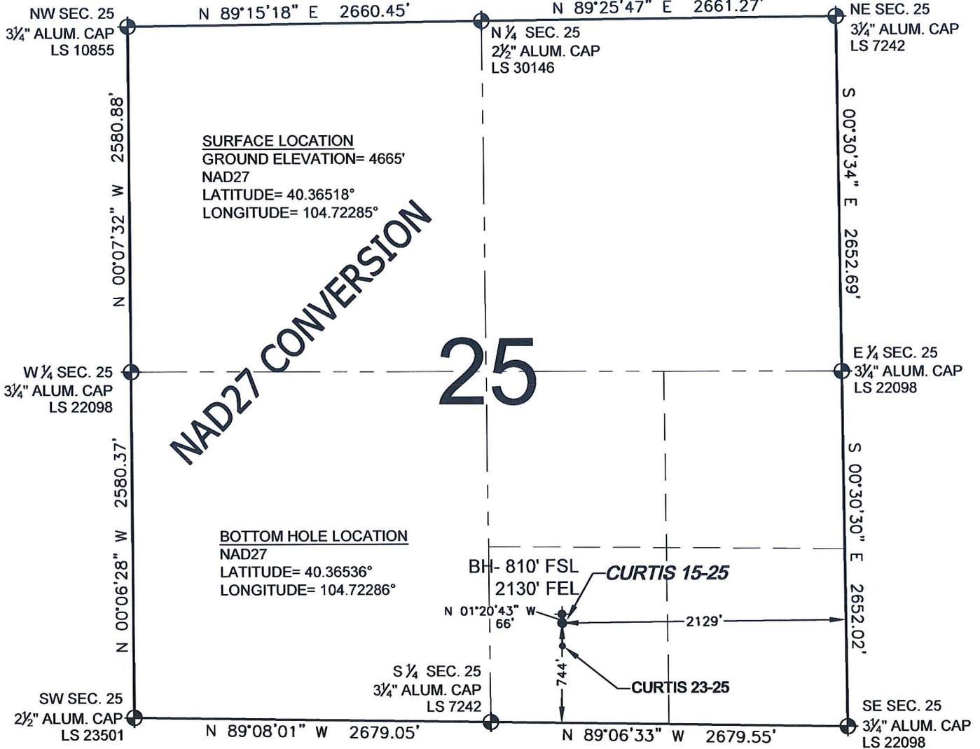
WELL CURTIS 15-25 TO BE LOCATED 744' FSL AND 2129' FEL, SECTION 25, T5N, R66W OF THE 6th P.M.
