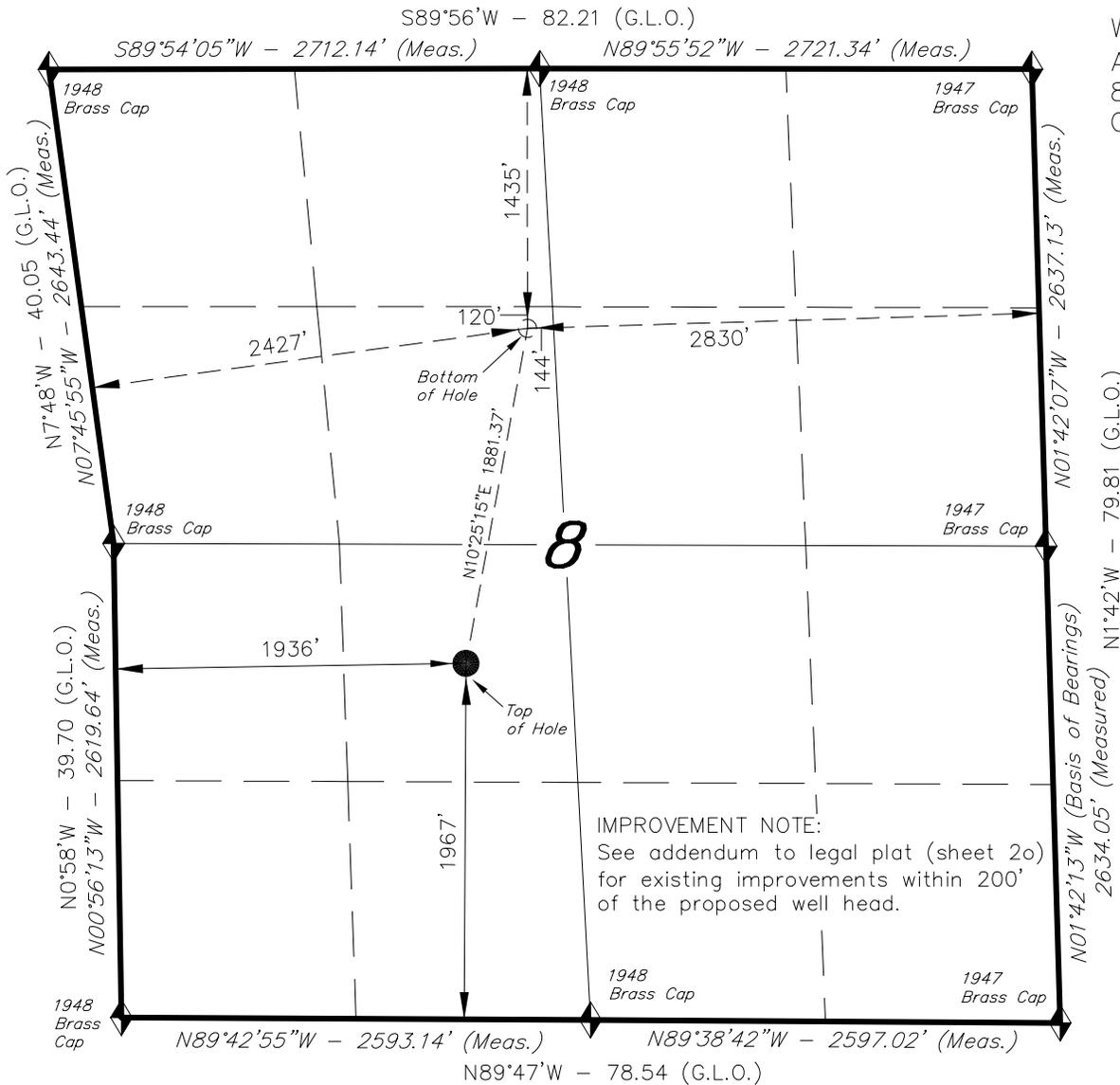
WELL LOCATION, GMR 8-6A1 (K8W), LOCATED AS SHOWN IN THE NE 1/4 SW 1/4 OF SECTION 8, T7S, R93W, 6th P.M. GARFIELD COUNTY, COLORADO.
