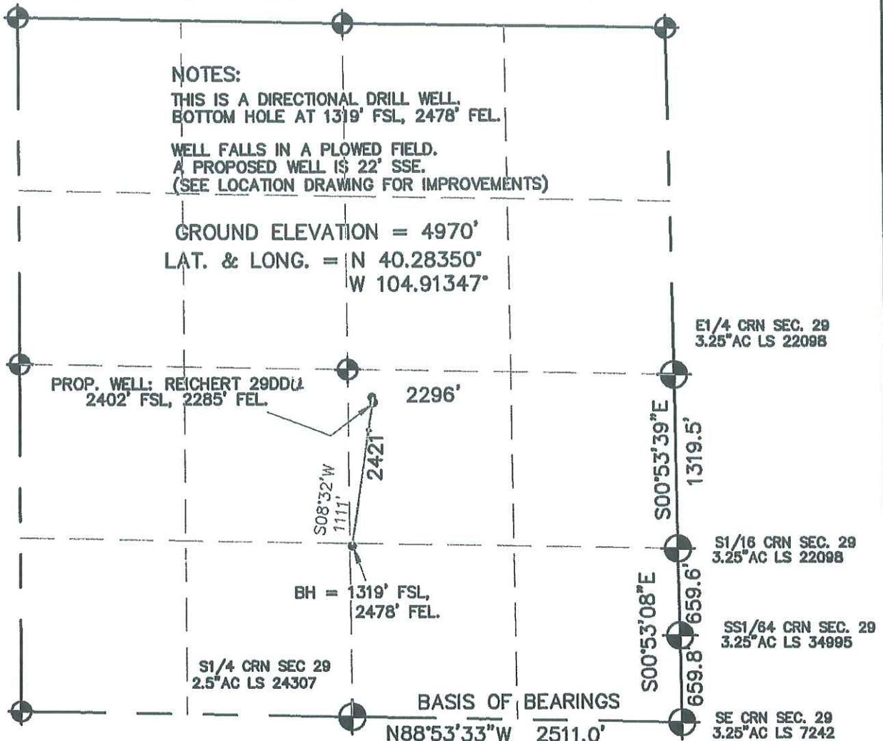
I HEREBY STATE TO UNIOIL THAT THIS WELL LOCATION CERTIFICATE FOR THE WELL REICHERT 29PDU IS LOCATED 2421' FSL & 2296' FEL, SEC. 29, T4N, R67W, 6PM.
