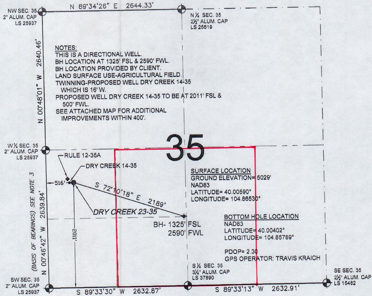
WELL DRY CREEK 23-35 TO BE LOCATED 2011' FSL AND 516' FWL, SECTION 35, T1N, R67W OF THE 6th P.M.
