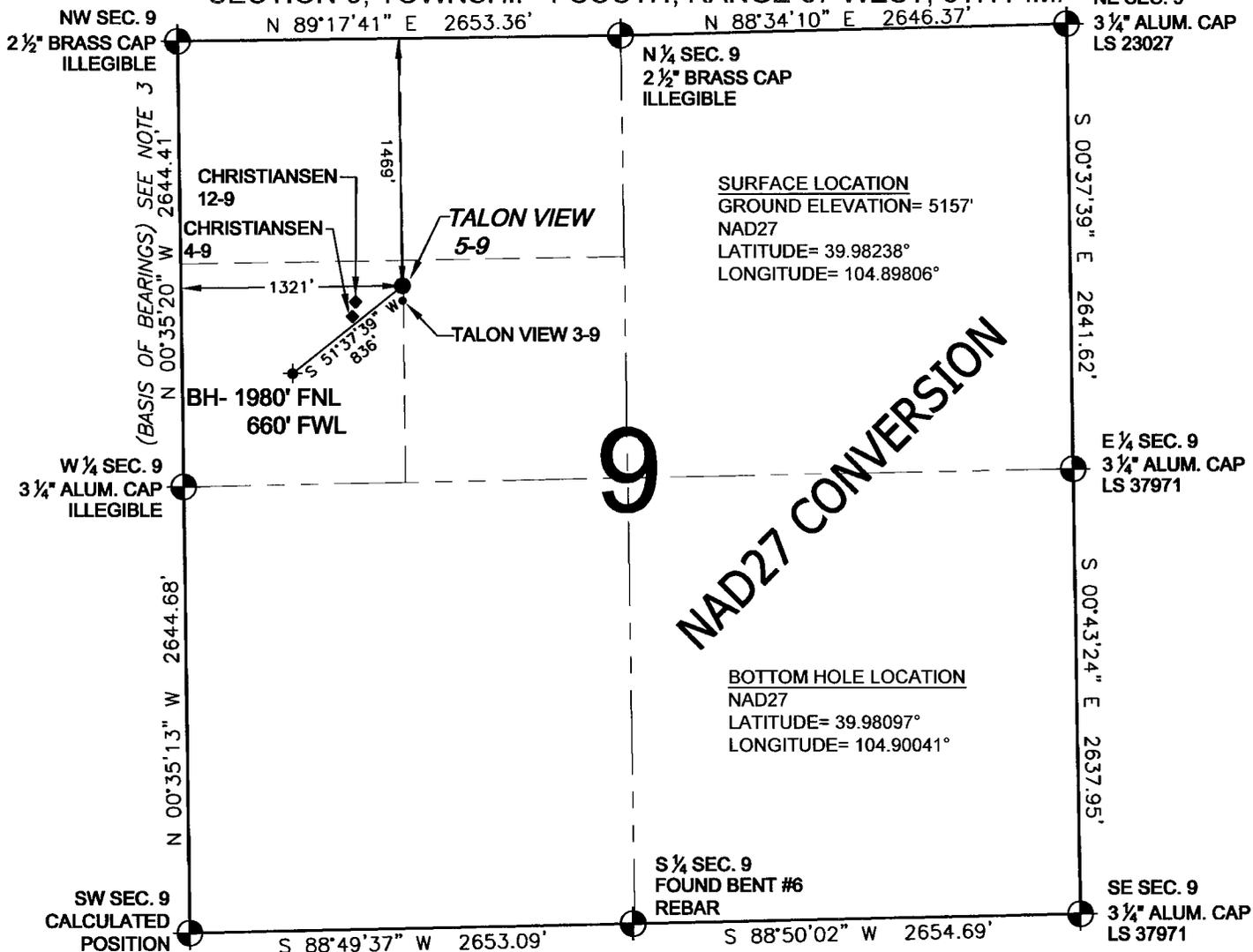
WELL TALON VIEW 5-9 TO BE LOCATED 1469' FNL AND 1321' FWL, SECTION 9, T1S, R67W OF THE 6th P.M.
