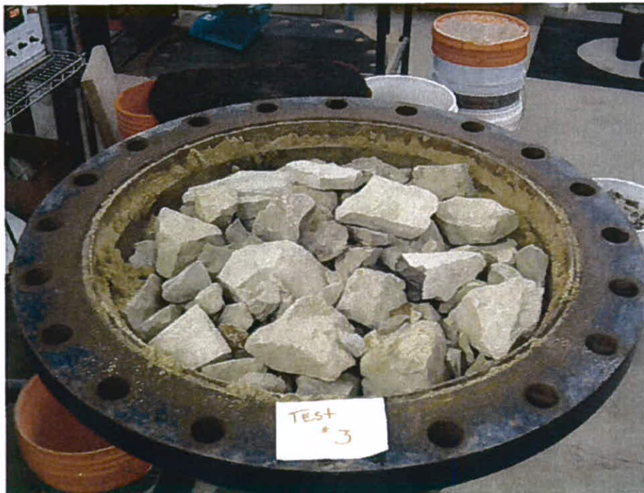
Example of the Roan Plateau shale placed over geosynthetic liner system
