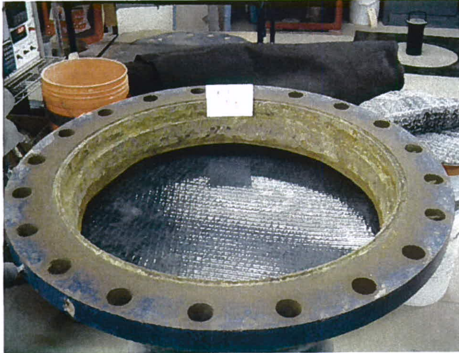
Test No. 3 geomembrane post exposure
