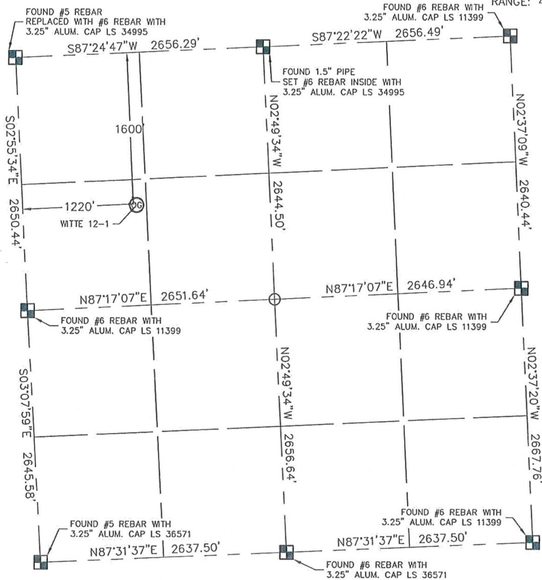
In accordance with a request from Dan Casper with Noble Energy Inc. King Surveyors Inc. has determined the surface location of the WITTE 12-1 to be 1600' from the NORTH line and 1220' from the WEST line as measured at right angles from the section line of Section 1, Township 2 South, Range 45 West of the Sixth Principal Meridian, County of Yuma, State of Colorado.
