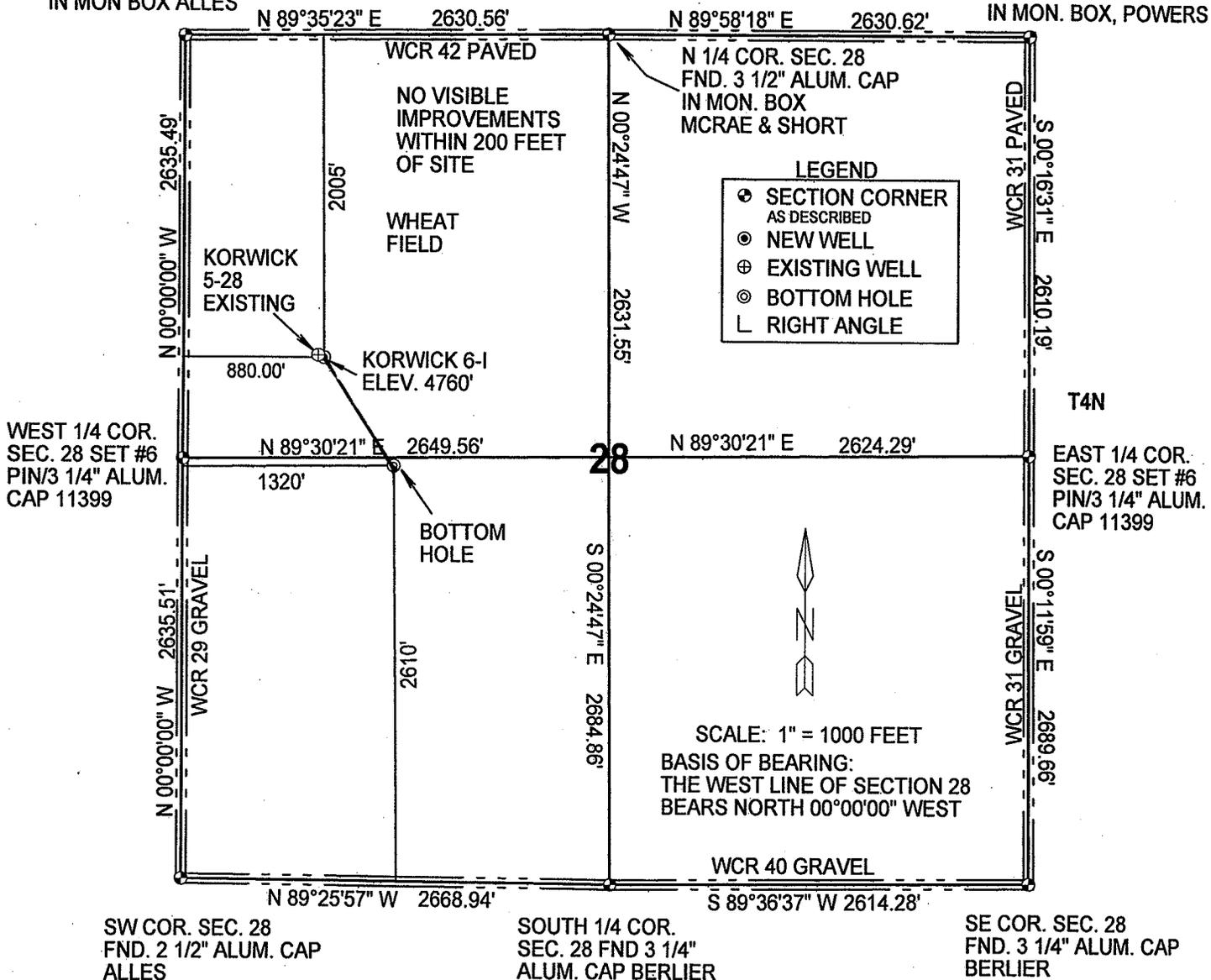
IN ACCORDANCE WITH A REQUEST FROM MERIT ENERGY COMPANY, THE UNDERSIGNED HAS DETERMINED THE LOCATION OF THE KORWICK 6-I WELL TO BE 880' FWL AND 2005' FNL, SECTION 28, TOWNSHIP 4 NORTH, RANGE 66 WEST OF THE 6TH PRINCIPAL MERIDIAN, WELD COUNTY, COLORADO. FIELD SURVEY DATE: AUGUST 20, 2008
