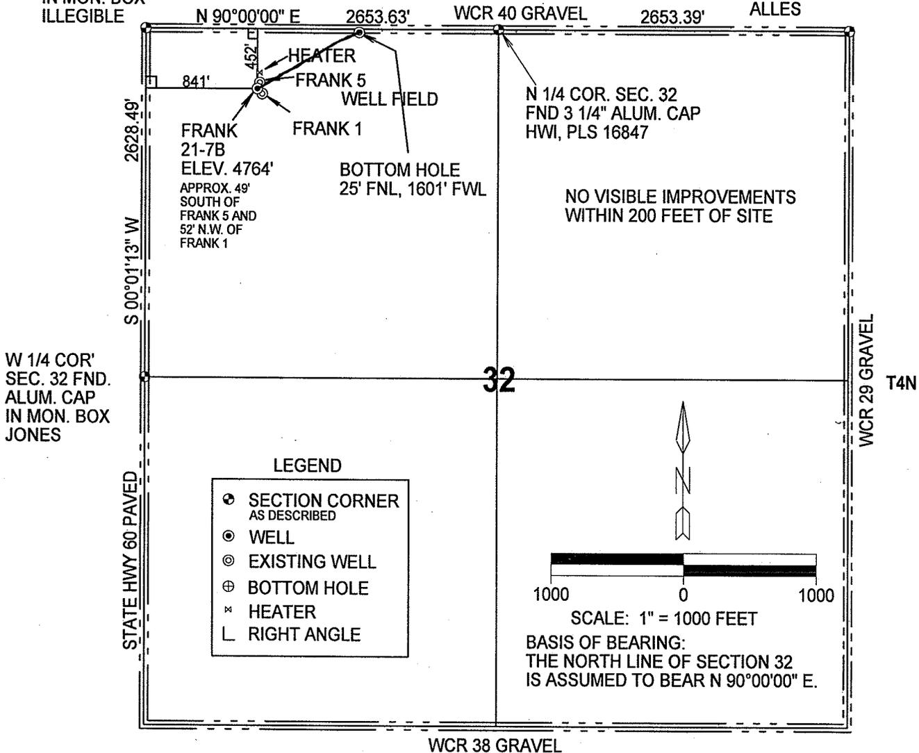
IN ACCORDANCE WITH A REQUEST FROM MERIT ENERGY COMPANY, THE UNDERSIGNED HAS DETERMINED THE LOCATION OF THE FRANK 21-7B WELL TO BE 841' FWL AND 452' FNL, SECTION 32, TOWNSHIP 4 NORTH, RANGE 66 WEST OF THE 6TH PRINCIPAL MERIDIAN, WELD COUNTY, COLORADO. FIELD SURVEY DATE: MAY 30, 2008.
