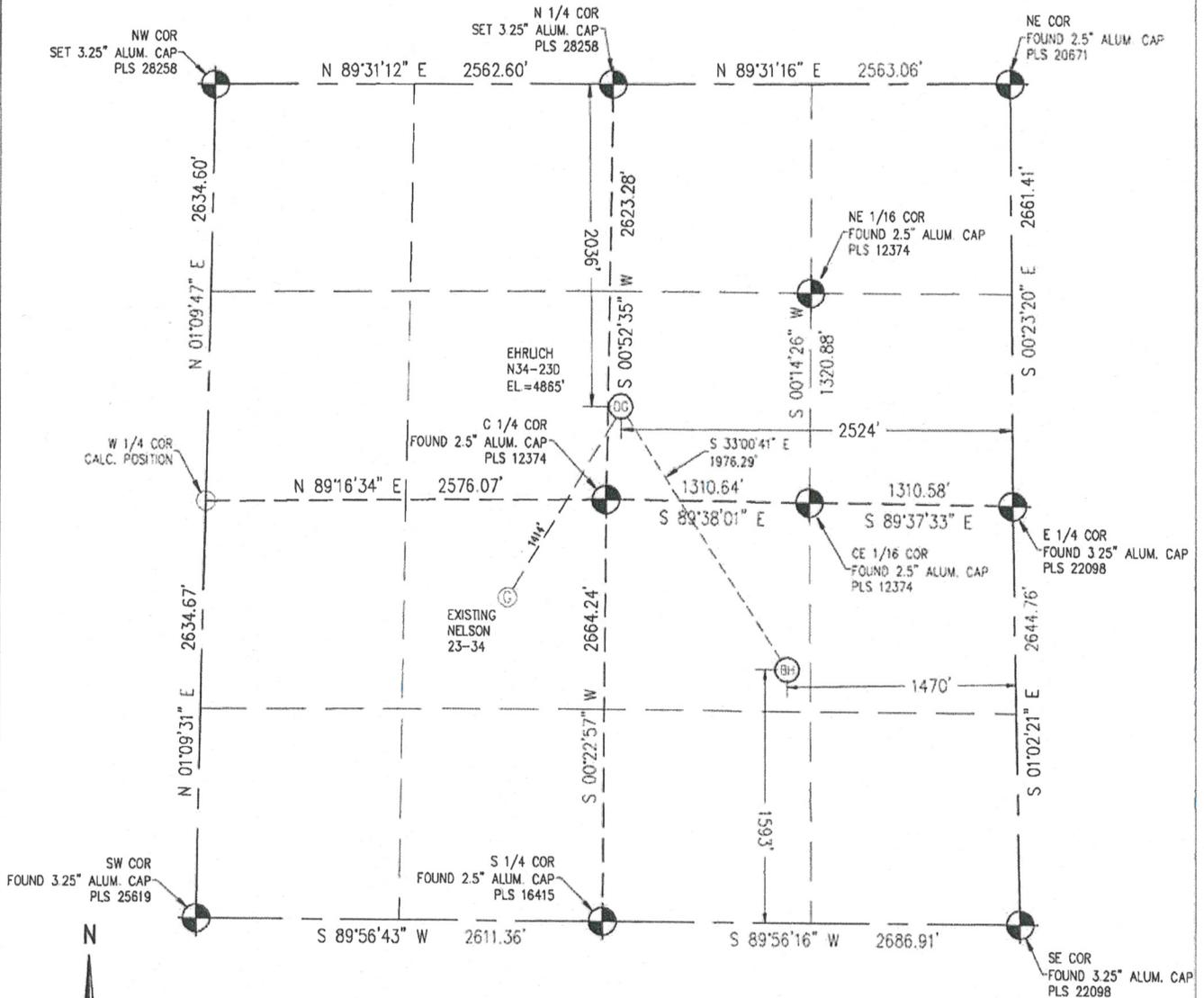
IN ACCORDANCE WITH A REQUEST FROM JOE MARTIN - NOBLE ENERGY INC, BASELINE ENGINEERING CORP. HAS DETERMINED THE LOCATION OF THE EHRLICH N34-23D TO BE 2036' FNL, 2524' FEL, AS MEASURED AT NINETY (90) DEGREES FROM THE SECTION LINE OF SECTION 34, TOWNSHIP 5 NORTH, RANGE 67 WEST AND THE BOTTOM HOLE LOCATION TO BE 1593' FSL AND 1470' FEL OF SECTION 34, TOWNSHIP 5 NORTH, RANGE 67 WEST, 6TH PRINCIPAL MERIDIAN, WELD COUNTY, COLORADO
