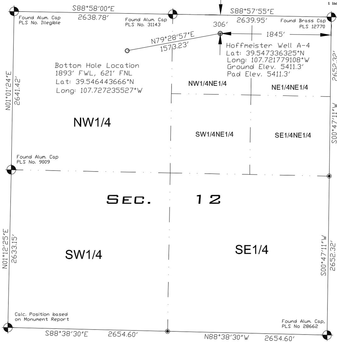
Bearings shown hereon are based upon RTK GPS observations.
