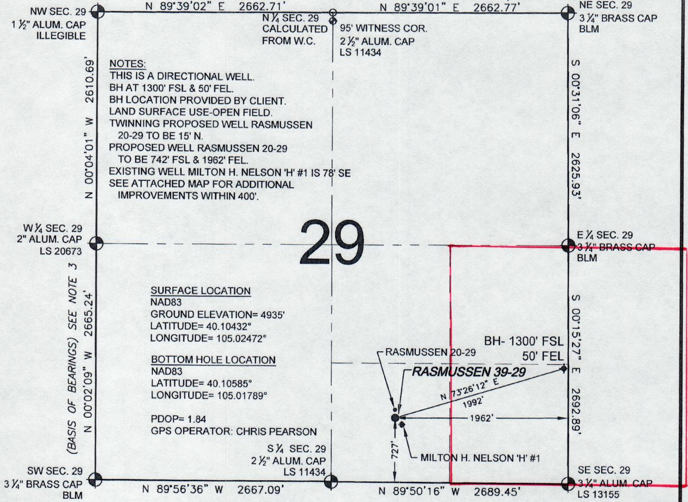
WELL RASMUSSEN 39-29 TO BE LOCATED 727' FSL AND 1962' FEL, SECTION 29, T2N, R68W OF THE 6th P.M.
