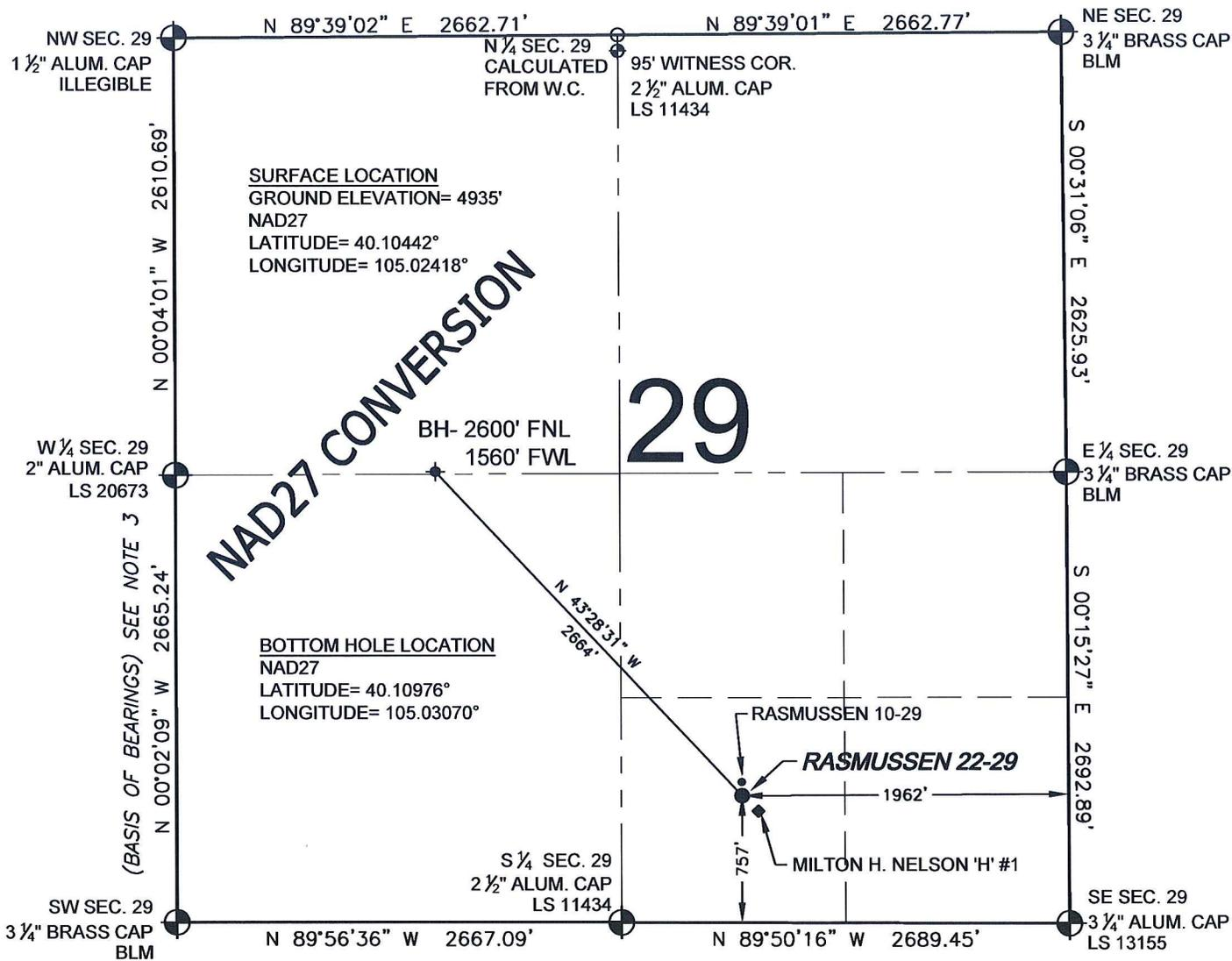
WELL RASMUSSEN 22-29 TO BE LOCATED 757' FSL AND 1962' FEL, SECTION 29, T2N, R68W OF THE 6TH P.M.
