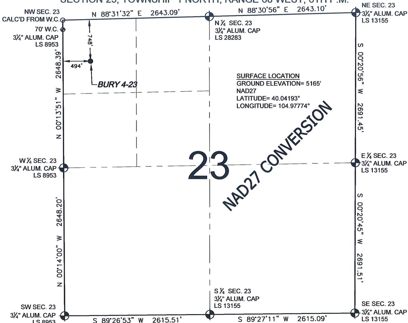
WELL **BURY 4-23** TO BE LOCATED 748' FNL AND 494' FWL, SECTION 23, T1N, R68W OF THE 6th P.M.
