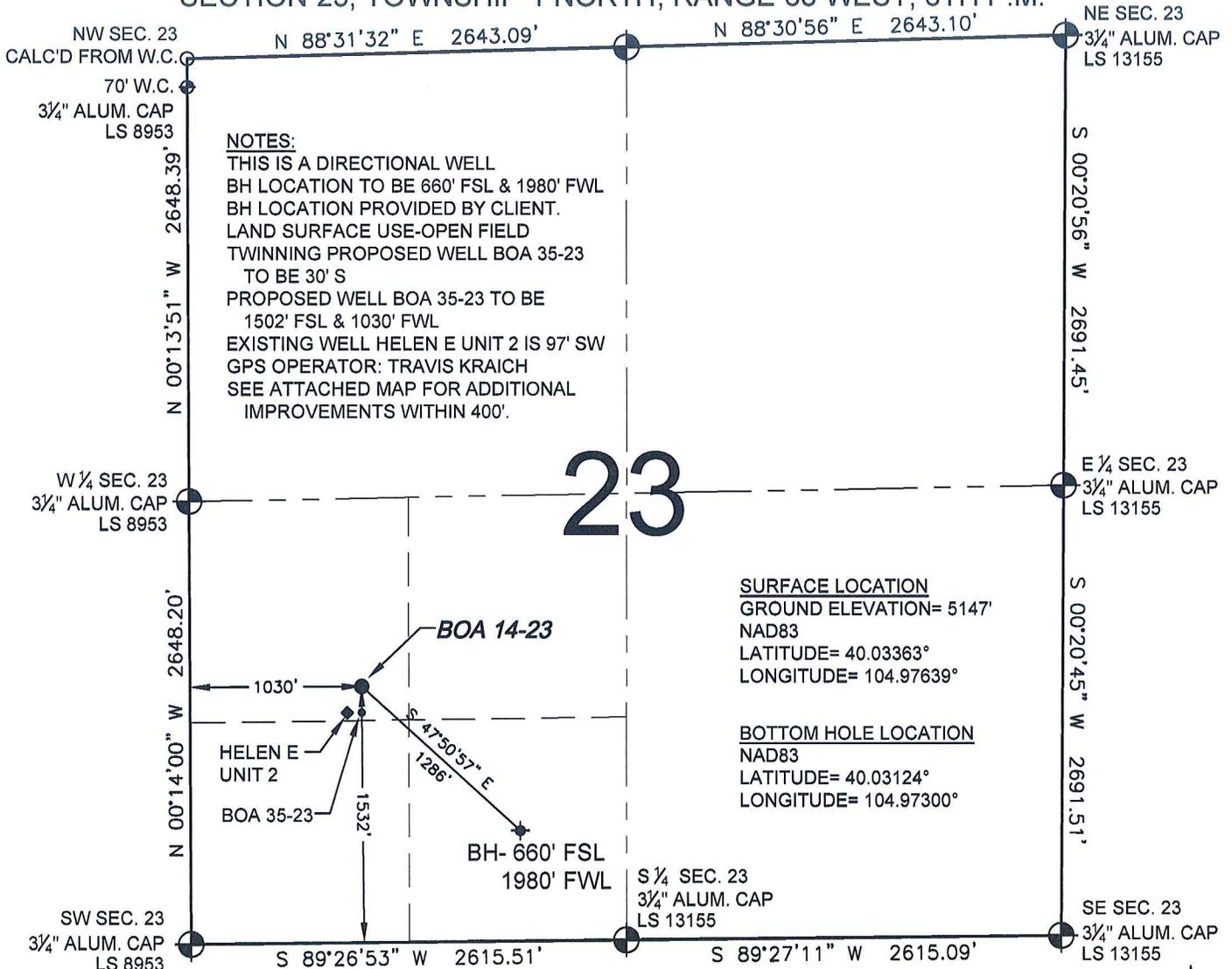
WELL **BOA 14-23** TO BE LOCATED 1532' FSL AND 1030' FWL, SECTION 23, T1N, R68W OF THE 6th P.M.
