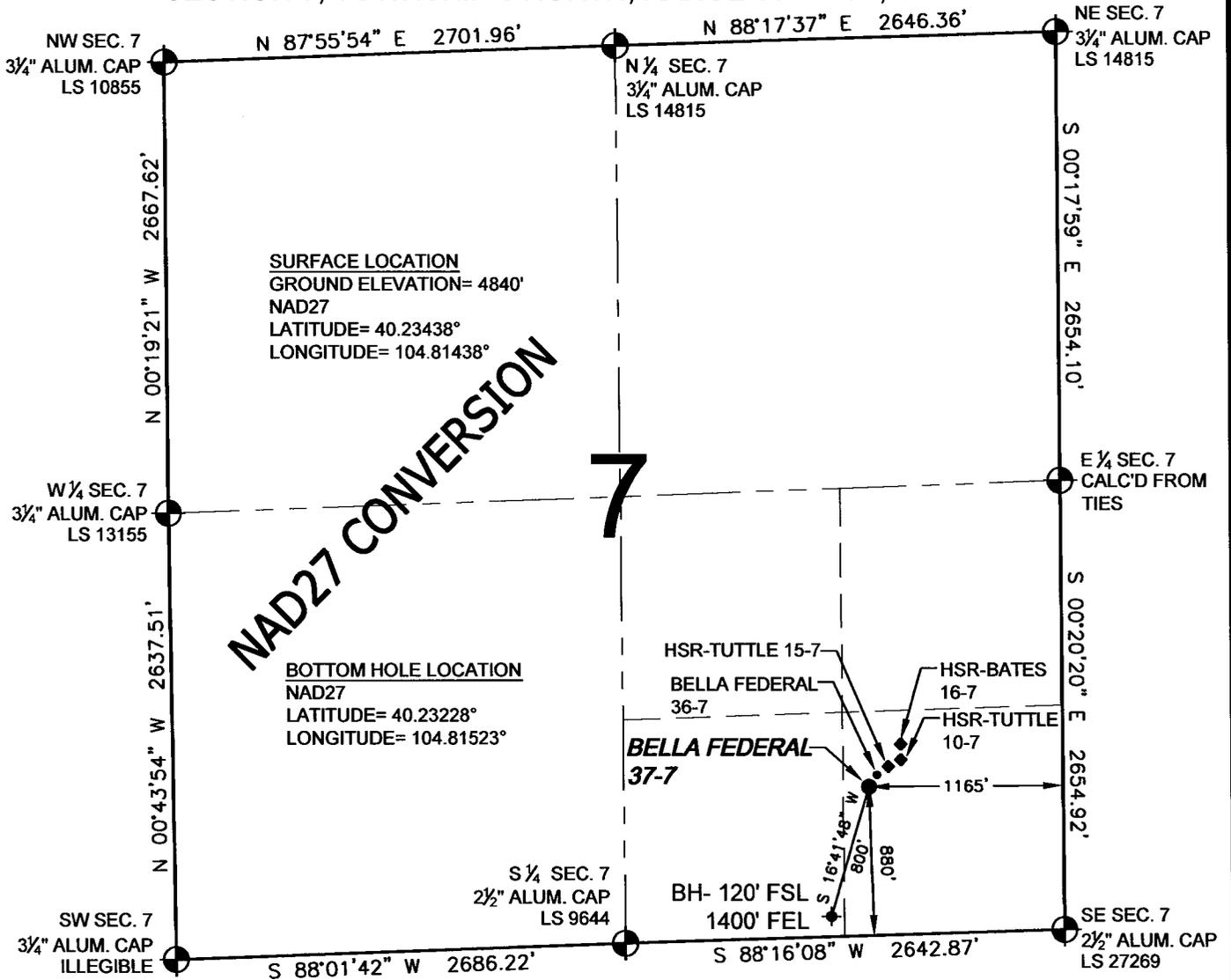
WELL **BELLA FEDERAL 37-7** TO BE LOCATED 880' FSL AND 1165' FEL, SECTION 7, T3N, R66W OF THE 6th P.M.
