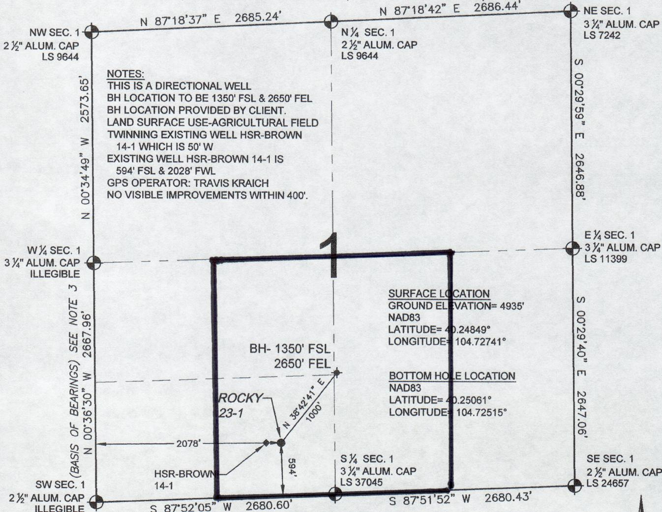
WELL ROCKY 23-1 TO BE LOCATED 594' FSL AND 2078' FWL, SECTION 1, T3N, R66W OF THE 6th P.M.
