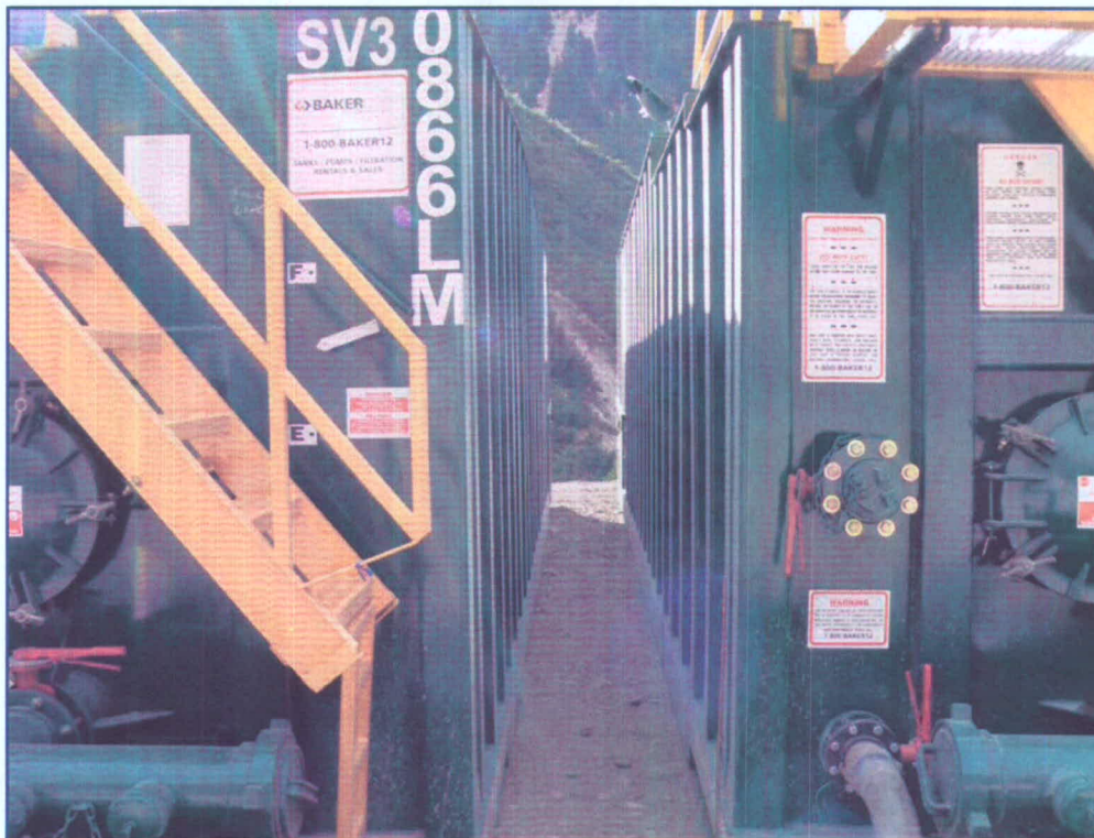
Close up view of two and one half foot spacing between frac tanks.
