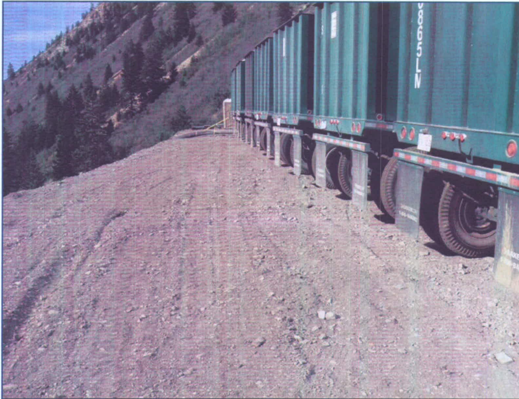
Back view of frac tanks showing minimum 3 foot spacing from edge of pad.
