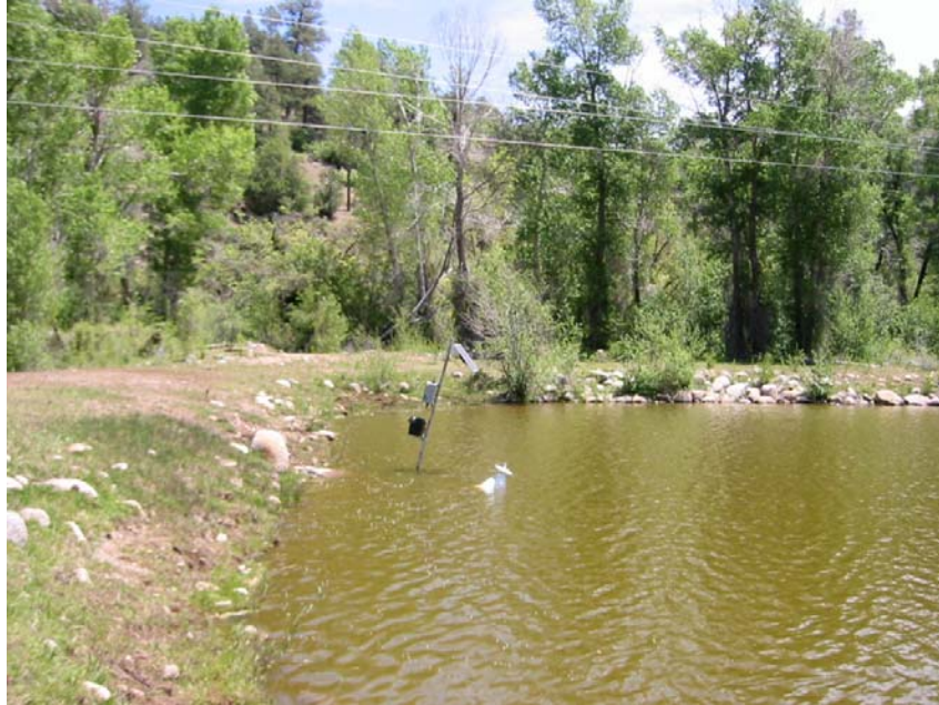
Methane seepage in the pond at Terry Palmer Ranch, View east. Note sinking flux chamber.
