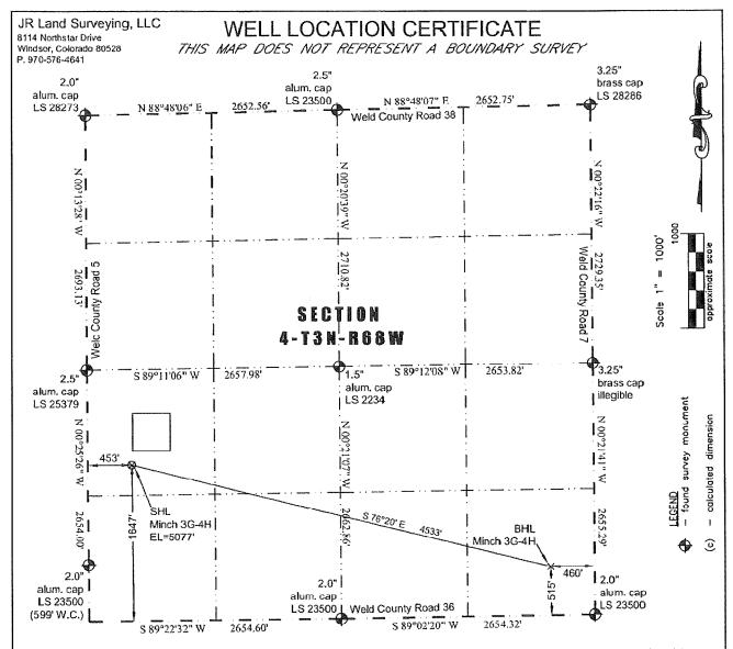
In accordance with a request from Jay Knutson of EnCana Oil & Gas (USA) Inc., JR Land Surveying, LLC has determined the location of the Minch 3G-4H well site to be SHL: 1647' FSL and 453' FWL, (BHL: 515' FSL and 460' FEL), as measured at ninety (90) degrees from the section lines of Section 4, Township 3 North, Range 68 West of the 6th Principal Meridian, Weld County Colorado.
