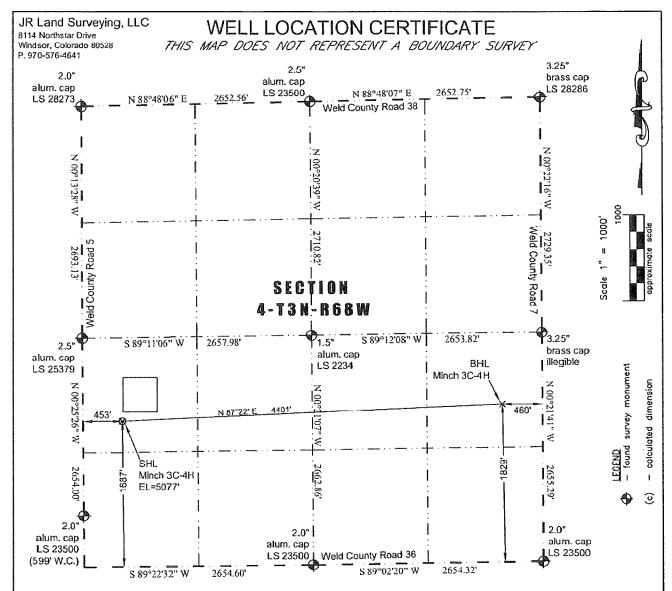
In accordance with a request from Jay Knutson of EnCana Oil & Gas (USA) Inc., JR Land Surveying, LLC has determined the location of the Minch 3C-4H well site to be SHL: 1687' FSL and 453' FWL, (BHL: 1829' FSL and 460' FEL), as measured at ninety (90) degrees from the section lines of Section 4, Township 3 North, Range 68 West of the 6th Principal Meridian, Weld County Colorado.
