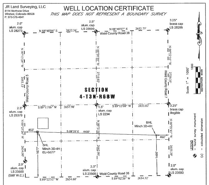
in accordance with a request from Jay Knutson of EnCana Oil & Gas (USA) Inc., JR Land Surveying, LLC has determined the location of the Minch 3D-4H well site to be SHL: 1677' FSL and 453' FWL, (BHL: 1495' FSL and 460' FEL), as measured at ninety (90) degrees from the section lines of Section 4, Township 3 North, Range 68 West of the 6th Principal Meridian, Weld County Colorado.
