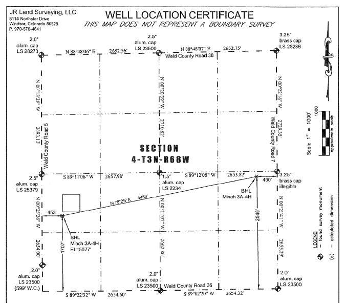
In accordance with a request from Jay Knutson of EnCana Oil & Gas (USA) Inc., JR Land Surveying, LLC has determined the location of the Minch 3A-4H well site to be SHL: 1707 FSL and 453 FWL, (BHL: 2546 FSL and 460 FEL), as measured at ninety (90) degrees from the section lines of Section 4, Township 3 North, Range 68 West of the 6th Principal Meridian, Weld County Colorado.
