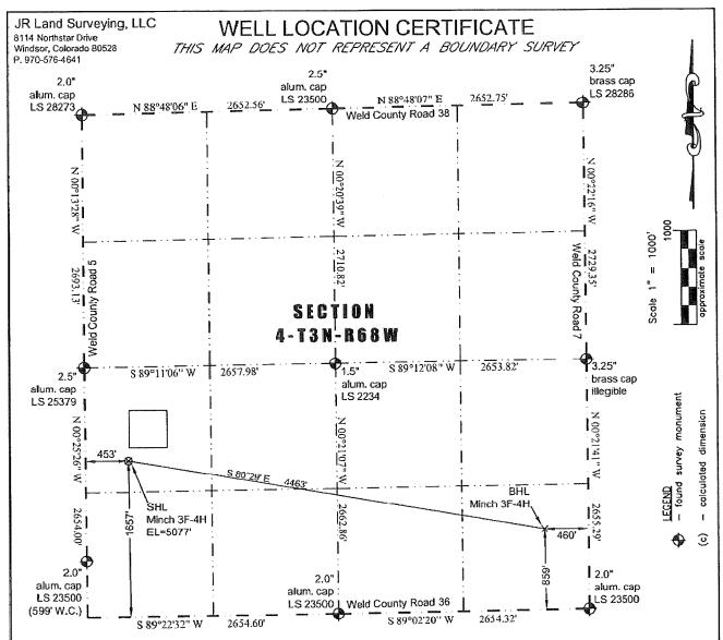
In accordance with a request from Jay Knutson of EnCana Oil & Gas (USA) Inc., JR Land Surveying, LLC has determined the location of the Minch 3F-4H well site to be SHL: 1657' FSL and 453' FWL, (BHL: 859' FSL and 460' FEL), as measured at ninety (90) degrees from the section lines of Section 4, Township 3 North, Range 68 West of the 6th Principal Meridian, Wold County Colorado.
