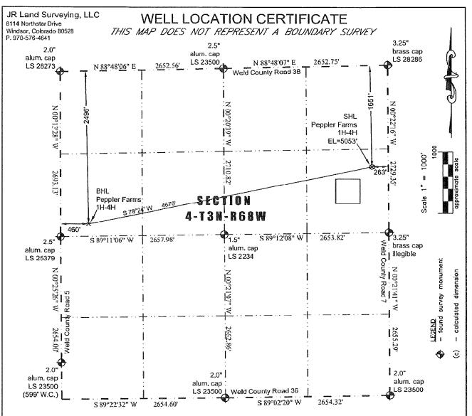
In accordance with a request from Jay Knutson of EnCana Oil & Gas (USA) Inc., JR Land Surveying, LLC has determined the location of the Peppler Farms 1H-4H well site to be SHL: 1651' FNL and 263' FEL, (BHL: 2496' FNL and 460' FWL), as measured at ninety (90) degrees from the section lines of Section 4, Township 3 North, Range 68 West of the 6th Principal Meridian, Weld County Colorado.
