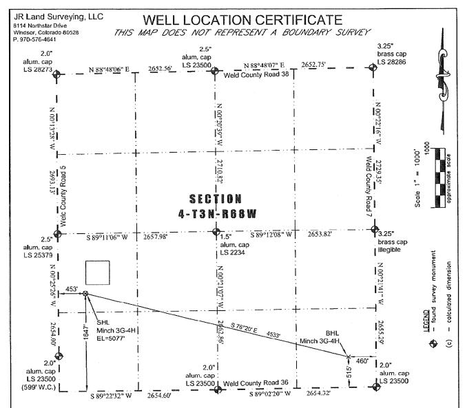
In accordance with a request from Jay Knutson of EnCana Oil & Gas (USA) Inc., JR Land Surveying, LLC has determined the location of the Minch 3G-4H well site to be SHL: 1647' FSL and 453' FWL, (BHL: 515' FSL and 460' FEL), as measured at ninety (90) degrees from the section lines of Section 4, Township 3 North, Range 68 West of the 6th Principal Meridian, Weld County Colorado.
