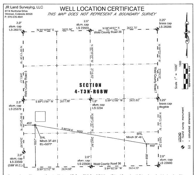
In accordance with a request from Jay Knutson of EnCana Oil & Gas (USA) Inc., JR Land Surveying, LLC has determined the location of the Minch 3F-4H well site to be SHL: 1657' FSL and 453' FWL, (BHL: 859' FSL and 460' FEL), as measured at ninety (90) degrees from the section lines of Section 4, Township 3 North, Range 68 West of the 6th Principal Meridian, Weld County Colorado.
