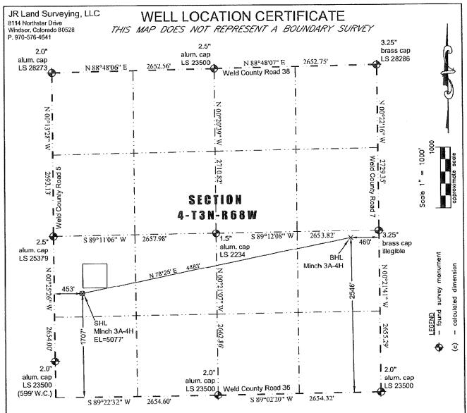
In accordance with a request from Jay Knutson of EnCana Oil & Gas (USA) Inc., JR Land Surveying, LLC has determined the location of the Minch 3A-4H well site to be SHL: 1707' FSL and 453' FWL, (BHL: 2546' FSL and 460' FEL), as measured at ninety (90) degrees from the section lines of Section 4, Township 3 North, Range 68 West of the 6th Principal Meridian, Wold County Colorado.
