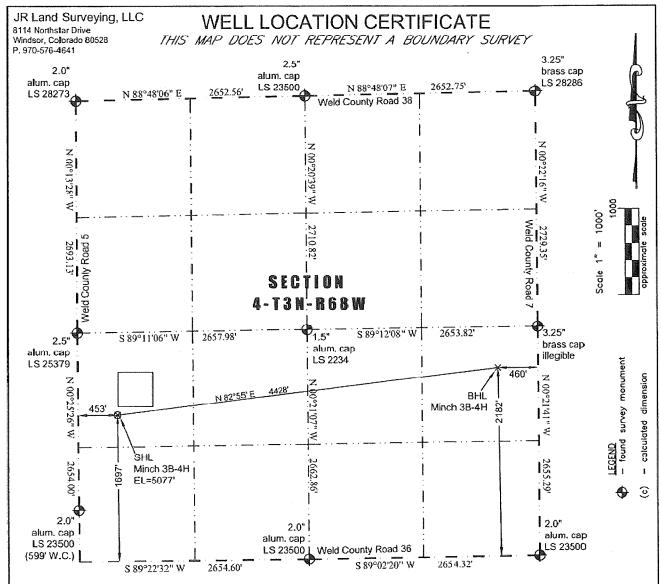
In accordance with a request from Jay Knutson of EnCana Oil & Gas (USA) Inc., JR Land Surveying, LLC has determined the location of the Minch 3B-4H well site to be SHL: 1697' FSL and 453' FWL, (BHL: 2182' FSL and 460' FEL), as measured at ninety (90) degrees from the section lines of Section 4, Township 3 North, Range 68 West of the 6th Principal Meridian, Weld County Colorado.
