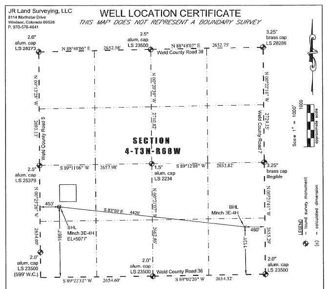
In accordance with a request from Jay Knutson of EnCana Oil & Gas (USA) Inc., JR Land Surveying, LLC has determined the location of the Minch 3E-4H well site to be SHL: 1667' FSL and 453' FWL, (BHL: 1131' FSL and 460' FEL), as measured at ninety (90) degrees from the section lines of Section 4, Township 3 North, Range 68 West of the 6th Principal Medidian, Weld County Colorado.
