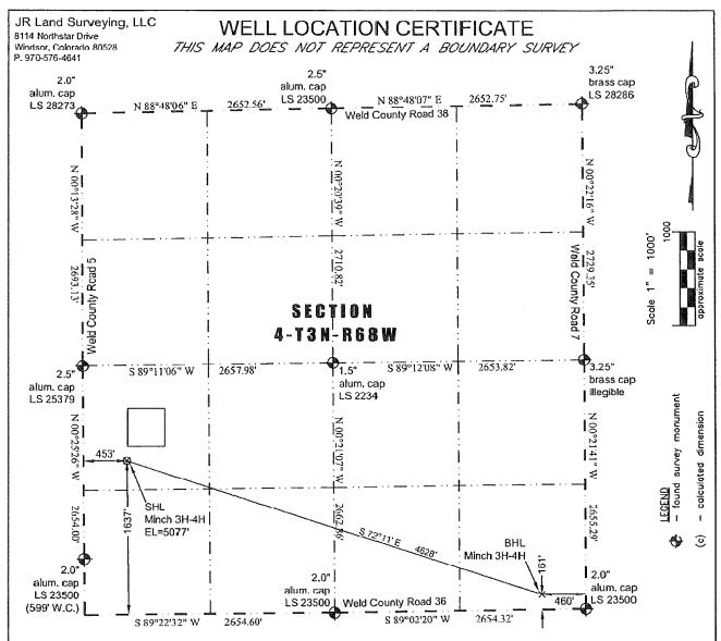
In accordance with a request from Jay Knutson of EnCana Oil & Gas (USA) Inc., JR Land Surveying, LLC has determined the location of the Minch 3H-4H well site to be SHL: 1637' FSL and 453' FWL, (BHL: 161' FSL and 460' FEL), as measured at ninety (90) degrees from the section lines of Section 4, Township 3 North, Range 68 West of the 6th Principal Meridian, Weld County Colorado,
