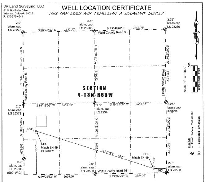
In accordance with a request from Jay Knutson of EnCana Oil & Cas (USA) Inc., JR Land Surveying, LLC has determined the location of the Minch 3H-4H well site to be SHL: 1637 FSL and 453' FWL, (BHL: 161' FSL and 460' FEL), as measured at ninety (90) degrees from the section lines of Section 4, Township 3 North, Range 68 West of the 6th Principal Meridian, Weld County Colorado.
