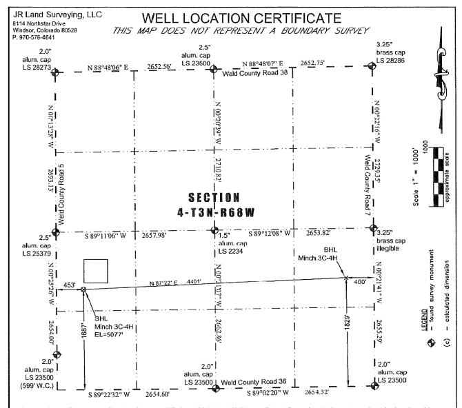
In accordance with a request from Jay Knutson of EnCana Oil & Gas (USA) Inc., JR Land Surveying, LLC has determined the location of the Minch 3C-4H well site to be SHL: 1687' FSL and 453' FWL, (BHL: 1829' FSL and 460' FEL), as measured at ninety (90) degrees from the section lines of Section 4, Township 3 North, Range 68 West of the 6th Principal Meridian, Weld County Colorado.
